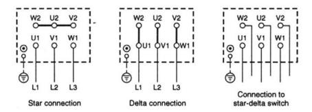
For special voltages and the like, different connections will be noted on the motor nameplate beside the voltage.
