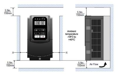
X = 1.18" (30mm) for inverter ratings up to 18.5kW X = 1.96" (50mm) for inverter ratings 22kW or higher
