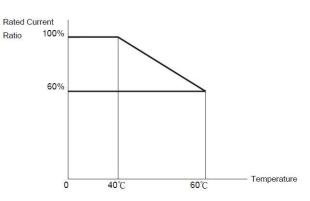
Note: User needs to adjust the inverter rated current depending on ambient temperature to ensure the appropriate industrial application  $\frac{1}{2}$
