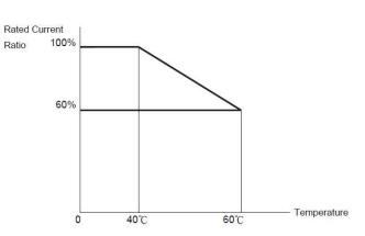
Note: User needs to adjust the inverter rated current depending on ambient temperature to ensure the appropriate industrial application  ${\bf r}$
