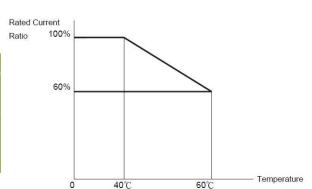
Note: User needs to adjust the inverter rated current depending on ambient temperature to ensure the appropriate industrial application
