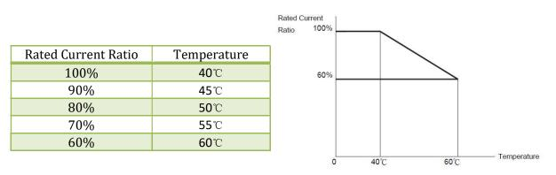
Note: User needs to adjust the inverter rated current depending on ambient temperature to ensure the appropriate industrial application
