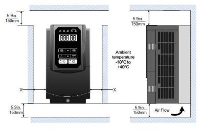
X = 1.18" (30mm) for inverter ratings up to 18.5kW X = 1.96" (50mm) for inverter ratings 22kW or higher
