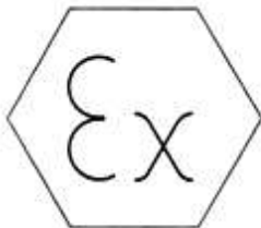
ENLARGED DETAIL OF EU EXPLOSIVE ATMOSPHERE SYMBOL
