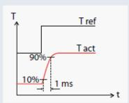
Closed and open loop: 100% torque step rise time = 1 ms.
