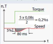
Closed loop = 0.2%sec (100% load step) Open loop = 0.4%sec (100% load step) Torque control dynamic accuracy:
