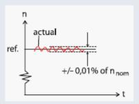
$\begin{aligned} &\text{Closed loop} = 0.01\% \text{ of } n_{\text{nom}}. \\ &\text{Open loop} = 0.1\% \text{ of } n_{\text{nom}}. \end{aligned}$
