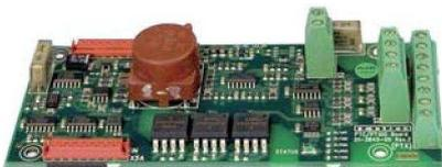
1 PTC isolated input conforming to DIN 44081/44082.
