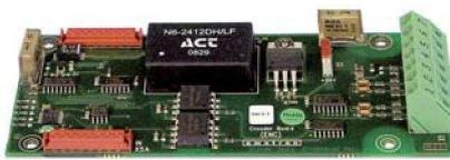
Differential encoder input suitable for 5 V (TTL) or 24 V (HTL) incremental encoders, range 5-16384 pulses/revolution. Inputs min 9 k $\Omega$ . Max frequency = 100 kHz. For single
