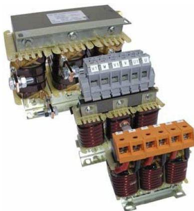
Output chokes (supplied separately) are recommended above app. 100 m cable length for all single drives. Consult your supplier in case of paralleled drives. Due to the switching of output voltage, high capacitive peak currents will run through the parasitic capacitances between the phases and to earth. Screened cables have more parasitic capacitances. Output chokes should be installed as close as possible to the drive output. Output chokes also
