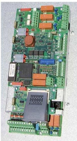
All drive boards are also available as coated, recommended e.g. for sewer pump applications (chlorine gases) or installations with occasional high humidity (if machine room installation or tropical climate). IEC60721-3-3 gases class 3C3, solid particles class 3S2.
