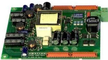
Built-in standby power supply board. To be connected to external 24 V AC/DC supply voltage. If the main power is switched off, the control board, control panel and the connected options, for example
