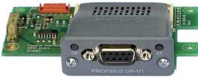
Fieldbus option module for Profibus DP or DP V1 communication. Use 9-pin D-sub connector.
