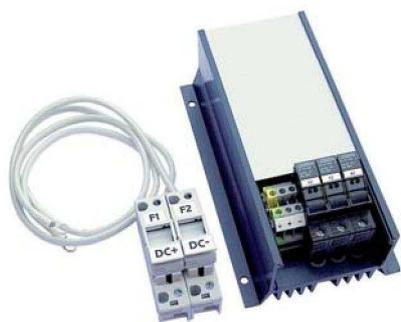
Together with the output choke, the overshoot clamp restricts the voltage and the dV/dt on the motor winding. For rated voltages 380 - 690 V. H x W x D = 250 x 145 x 95 mm
