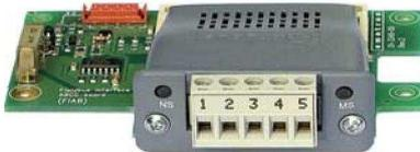
Fieldbus option module for DeviceNet communication. Baud rates: 125 - 500 kbits/s supported.
