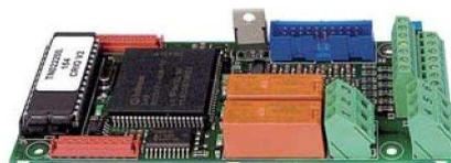
Crane option board to control hoist or travel motions. Inputs for joystick control: supporting 4-step, motor potentiometer or analog reference joystick types. Inputs for slow down and end limits switches (2+2). All 12 digital inputs 24 V/5 k $\Omega$  (8 - 24V) DC.
