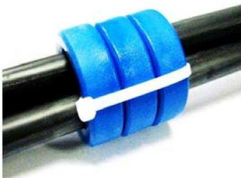
Common mode filters are mainly used to reduce common mode currents in motors (typically used with motors >size 280). Common mode filters can prevent damage of motor bearings. All three motor phases are to be routed through common mode filter rings. These filter can also be used to reduce EMC emissions in supply cables.
