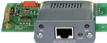
Industrial Ethernet option module for Modbus/TCP protocol. RJ45 type connector.
