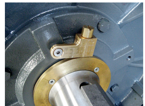
Rotor Grounding Brush fitted to a 280 Frame Motor.
